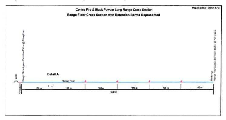
Detail 'A' - Cross Section of Retention Berms within Range Floor
